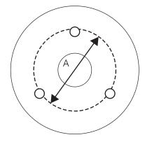
**3-LUG:** Diameter of virtual circle passing through center of all three bolt holes.
