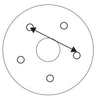
5-LUG: Back of one hole to the center of the second hole.
